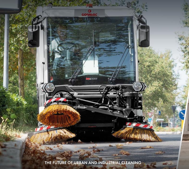
HP4000 is the powerful street sweeping machine with a green soul, designed to take cleaning to the next level, reducing waste and emissions. The rotating shaft with hammers with which the HP4000 is equipped allows large waste to be shredded into small pieces. The sweeping machine can therefore collect much more material than its competitors, filling the hopper completely.
